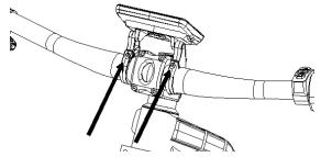
Adjust the headlight to the desired position, tighten the screws with a 4mm hex key
