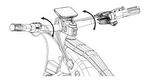
Set the handlebars into the mounting bracket and reattach the cap with the four hex bolts. Make any final adjustments and alignments then tighten the hex bolts so that the handlebars are secure. Check all the cables to ensure that they have not lost connection during the assembly.
