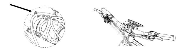
Cables can work loose and disconnect during shipping. Check all the cables to ensure they have not come loose. If a cable is loose, apply gentle pressure to each side to reconnect. If cables are completely disconnected, use the arrows on the side of the connector to align the pins before connecting. DAMAGE TO THE PINS CAUSED BY MISALIGNMENT WILL VOID THE WARRANTY
