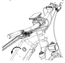
3. Place the charger in a flat, secure place and plug the charger into the battery's charging port, **before plugging into the power out**.
