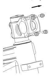
Orientate the handlebars so that the cables are not twisted and adjust the position.
